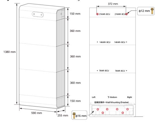
Figure 4-5 Dimensions for wall mounting
