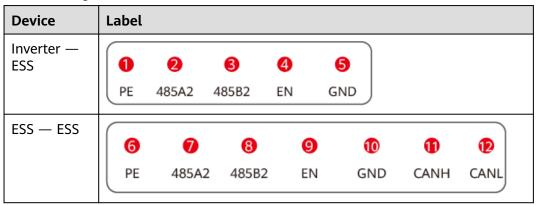
Figure 5-6 Network cable preparation
