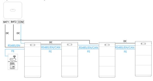
Figure 2-12 Connecting the ESSs to the inverter (4)
