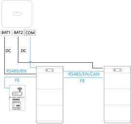
Figure 2-11 Connecting the ESSs to the inverter (3)
