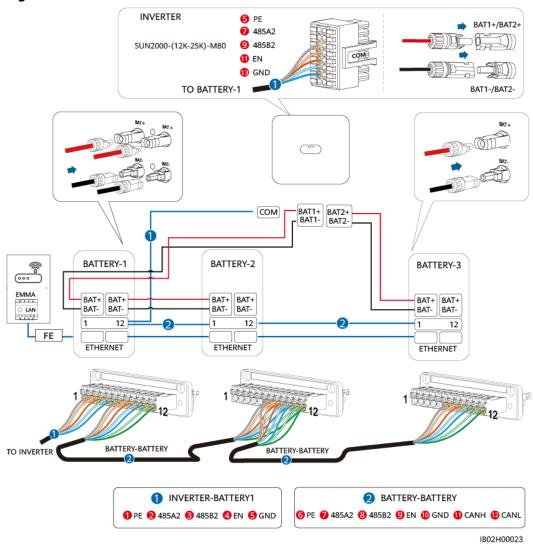
Figure 5-10 Inverter connected to three ESSs
