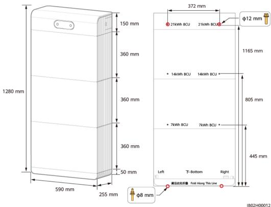
Figure 4-4 Dimensions for floor mounting
