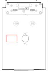
Figure 2-16 Nameplate position of the Energy Storage Module
