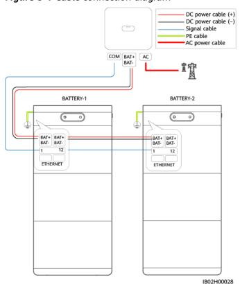
Figure 3-1 Cable connection diagram
