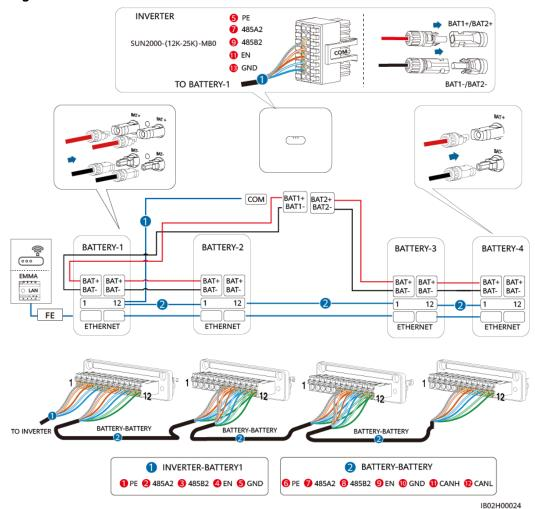
Figure 5-11 Inverter connected to four ESSs
