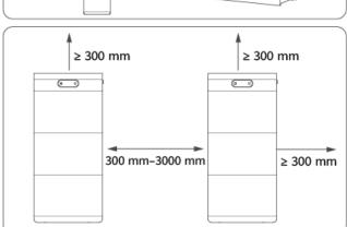
Figure 4-3 ESS installation requirements
